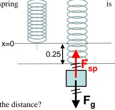
b) What mass would be required to stretch the spring three times the distance? 3xs or 15 kg since the mass is directly proportional to the displacement
