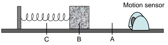
7. The diagram above shows a 2 kg block attached to a Hookean spring on a <u>frictionless</u> surface. The block experiences no net force when it is at position B. When the block is to the left of point B the spring pushes it to the right. When the block is to the right of point B, the spring pulls it to the left.
